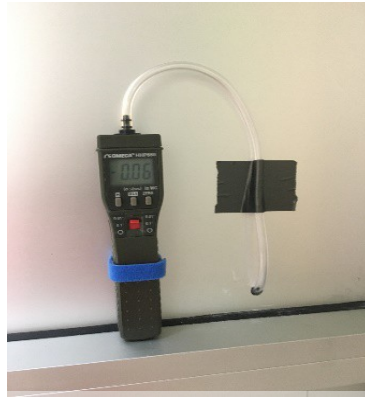
Pressure Sensor Requirement: -0.05" wc
