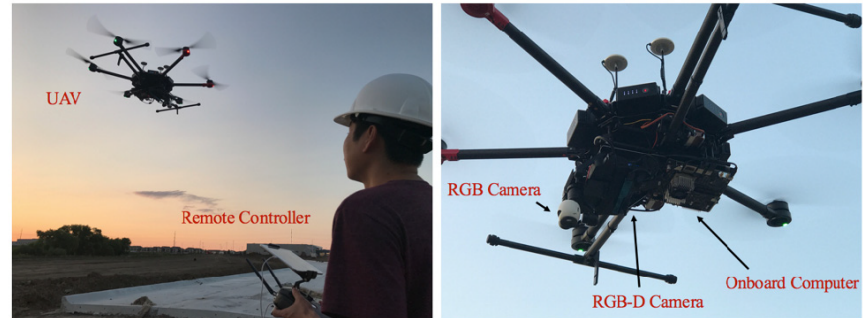
Figure 3. Experimental Setup: (a) UAV and on-site operator; (b) the attached positions of RGB camera, RGB-D camera and onboard computer on the craft
